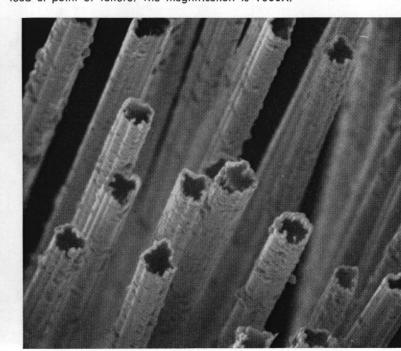
Nickel-coated fibers at 1000X magnification. The layer of nickel on
